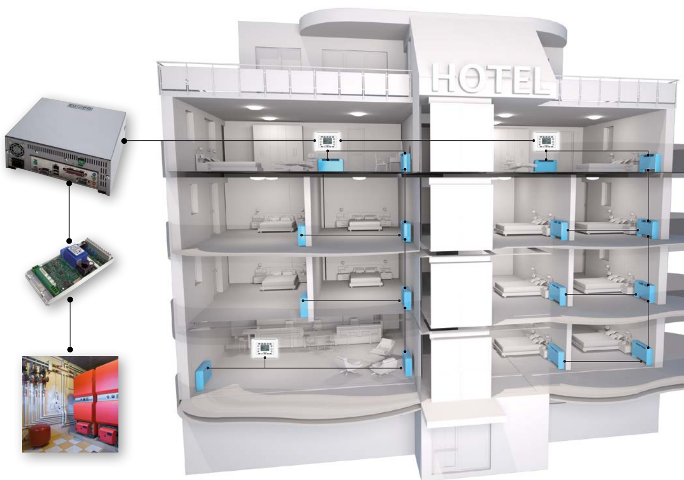
SUPERVISION SYSTEM WITH WEB SERVER-RS-485 (MAX. 128 UNITS DIRECTLY CONNECTED TO A SINGLE NET – MAX 8 NETS).
