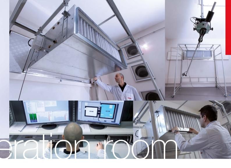
The two reverberating rooms have different dimensions: 84 and 227 m<sup>3</sup> respectively and are connected each other by an air duct.
