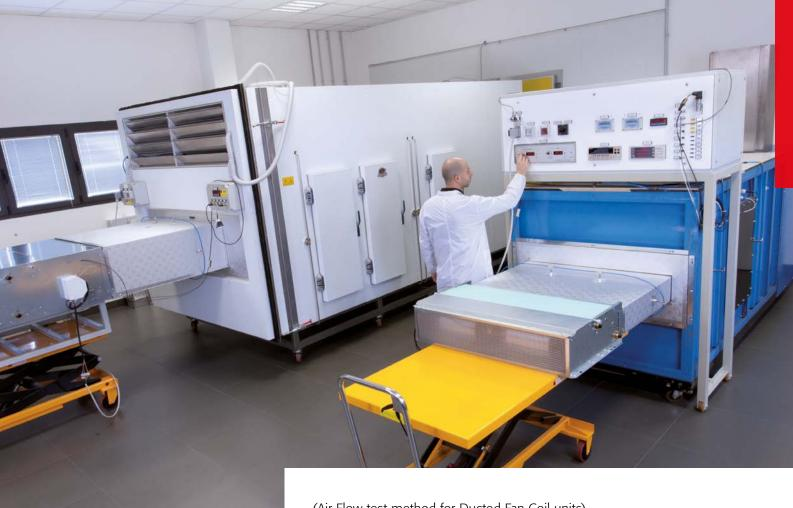
(Air Flow test method for Ducted Fan Coil units). The tunnel has been sized to ensure a correct measurement of the airflow from 120 m<sup>3</sup>/h to  $6000 \text{ m}^3$ /h.
